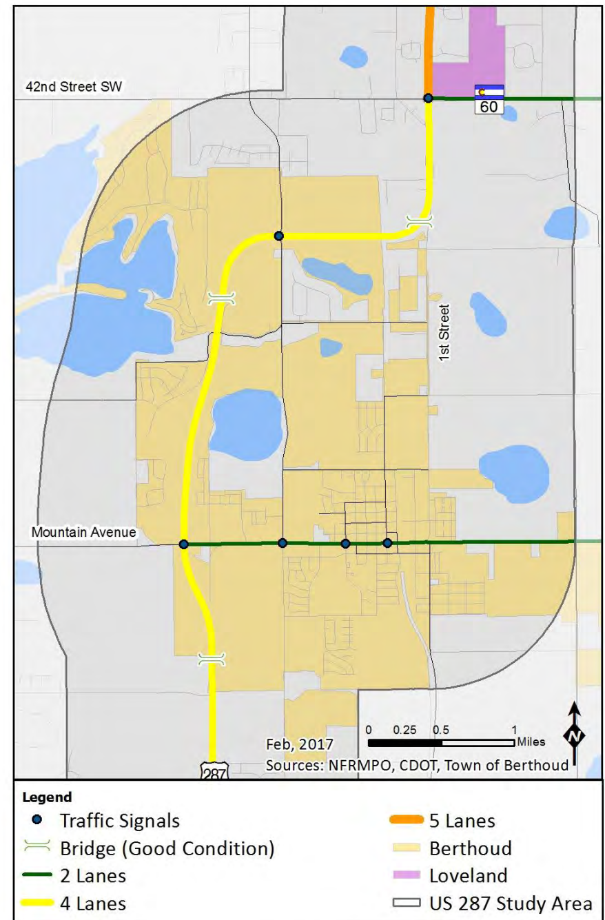
Figure 7-1 Berthoud Bridges, Number of Through Lanes, and Traffic Signals
