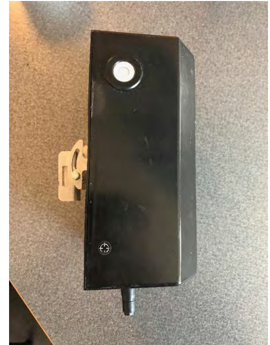
Figure 3: The Hi-Trac infrared counter can be set up to count all traffic by direction on shared-facilities, or can be paired with the Trax Cycles Plus to distinguish bikes from pedestrians.
