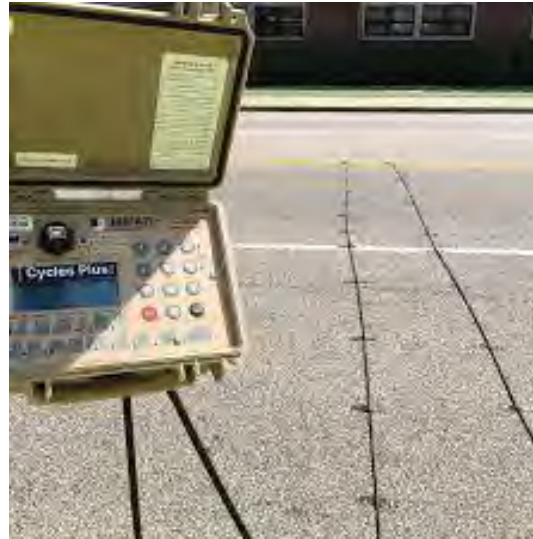
Figure 2: The Trax Cycles Plus tube counters that can be set up in various configurations to distinguish between mixed traffic on roads, or bike traffic alone on trails.
