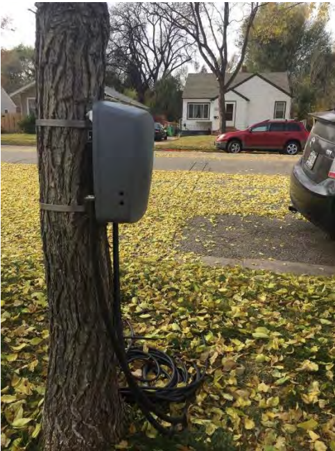
Figure 1: The NFRMPO has one tube/infrared combination counter that can be set up in various configurations to count bikes alone, pedestrians alone, or bikes and pedestrians together on shared or separate facilities
