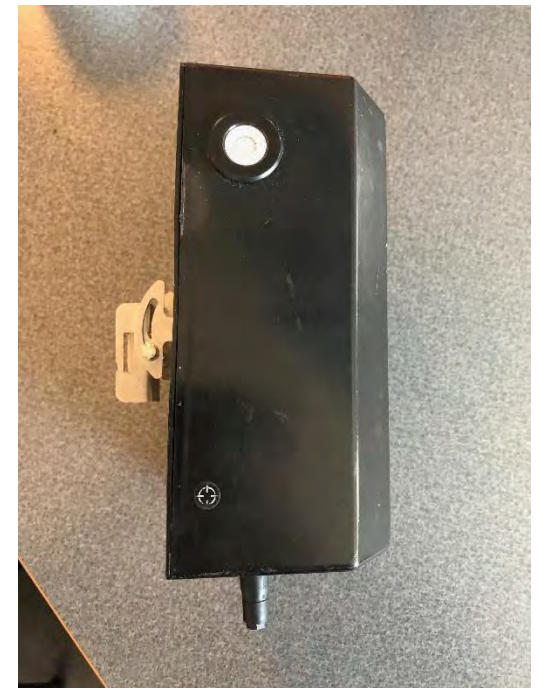
Figure 3: The NFRMPO has one infrared counter that can be set up to count total trail users by direction or can be paired with the tube counter to distinguish bikes from pedestrians
