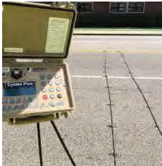
Figure 2: The NFRMPO has two tube counters that can be set up in various configurations to distinguish between mixed traffic on roads, or bike traffic alone on trails.
